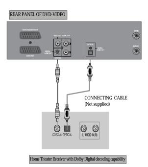
**1** Select either COAXIAL or OPTICAL to connect to amp of Dolby Digital.
